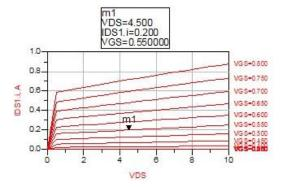
Figure 3. Graph of IV characteristics of transistor
