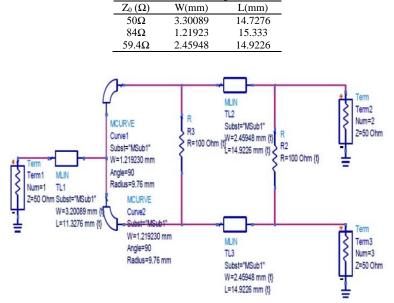
Figure 4. Schematic diagram of multi-section WDP
